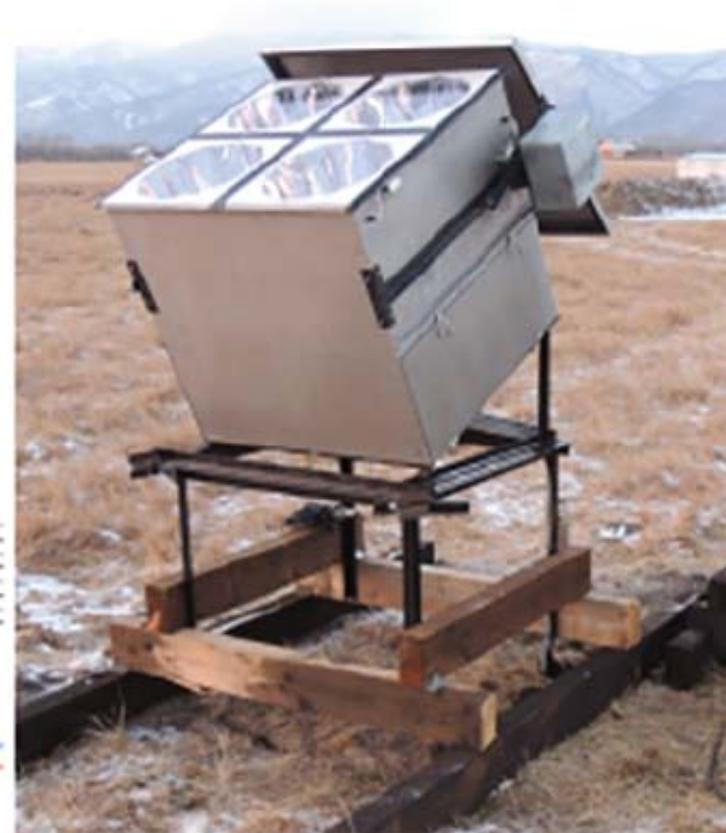
**Figure 2.** Schematic diagram of the Cherenkov container with the PMT of a Cherenkov detector of the TAIGA-HiSCORE array (left) and its photograph (right).
